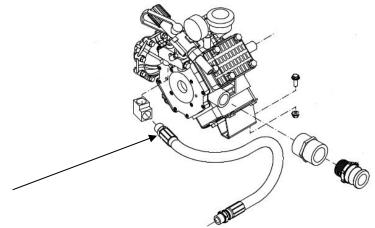
5. Remove and discard the old belt guard support bracket. Install new bracket designed to fit your new replacement pump. Attach this new bracket accordingly.
